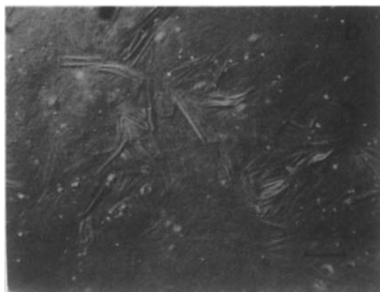
FIG. 3. Differential interference contrast photomicrographs of a ternary gel, T_2 , containing 1% cetostearyl alcohol before (a) and after (b) temperature cycling. Note the change in the amount of liquid crystalline network (1 division = 25 \mu m).
